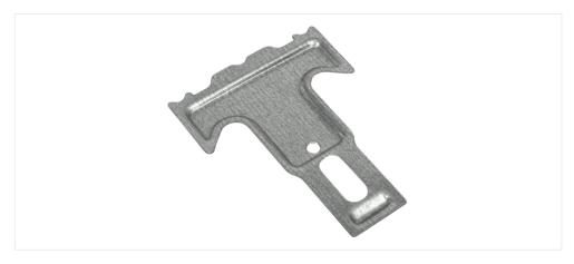
Single connector 60/27 Designed for attaching carrier profiles to the main profiles in a suspended ceiling. Applicable with a 60/27 ceiling profile.
