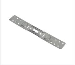
Accessory used as suspenders Ceiling System and adjustable bracket for Wall Lining System. Can be cut and bend according to the suspension height. Designed exclusively to be used with Ceiling System and Lining System. (Load bearing capacity class = 40 kg.)
